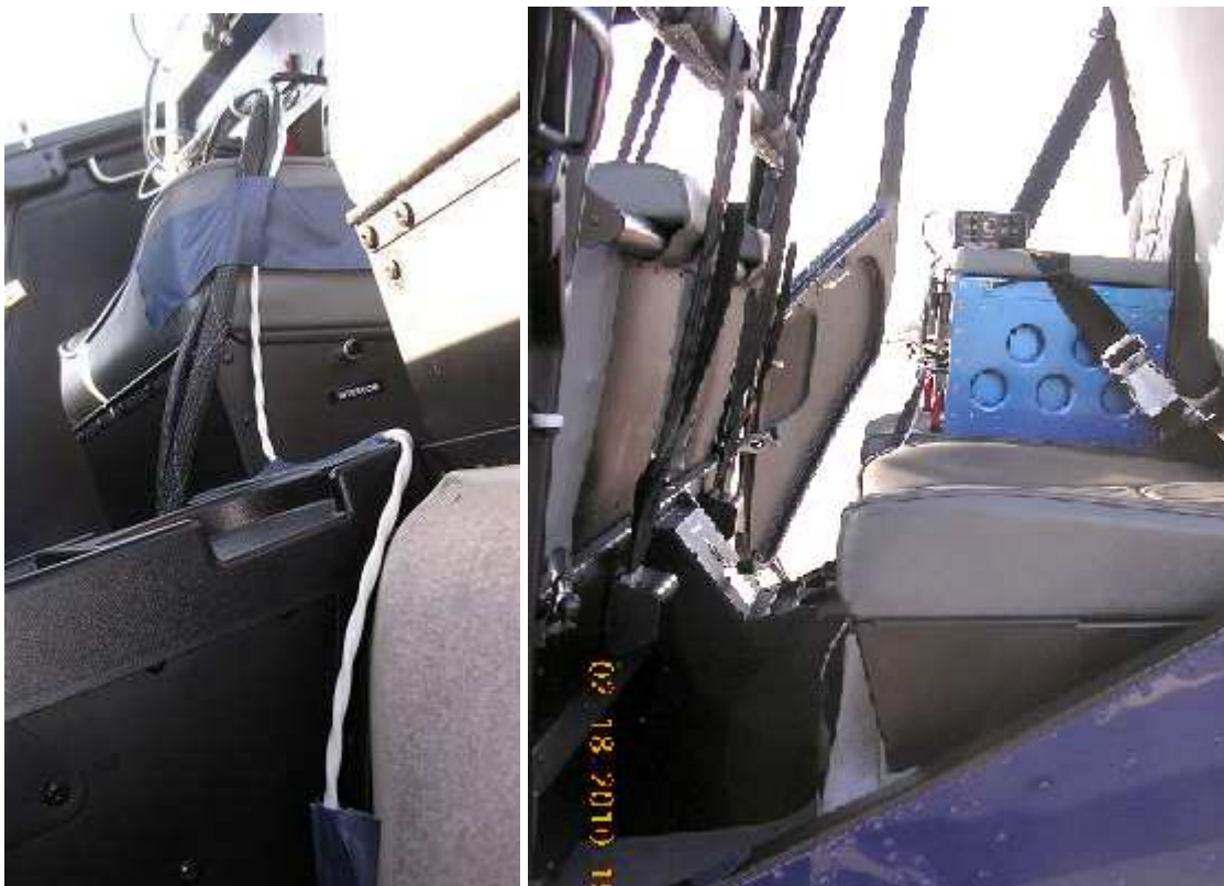
Figure B.1: Power Wire Routing
