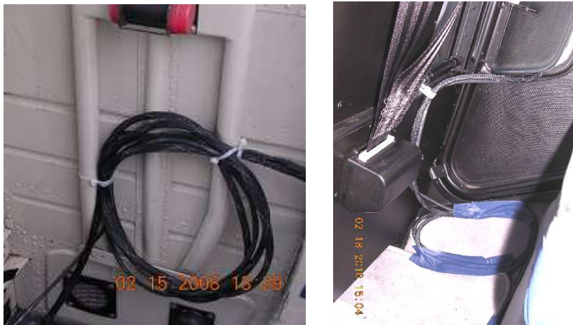
Figure 1.9, Interior Wiring Attachment
