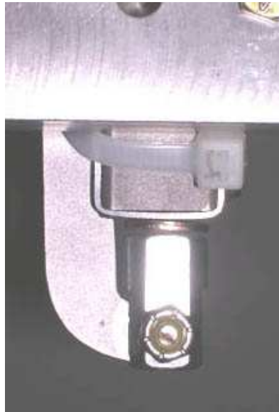
Figure 1.4: Clamp closed with zip tie
