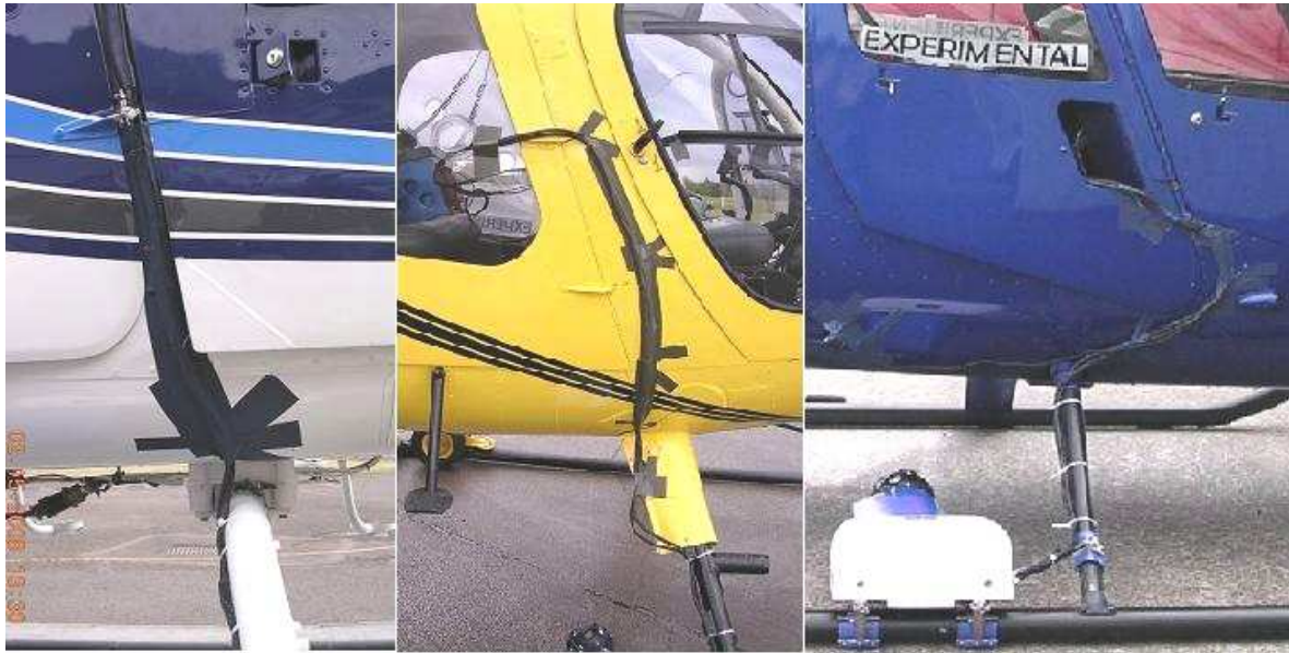
Figure 1.8, Exterior Wiring Attachment
